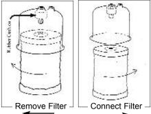
Step 7 Connect the housing top with bottom and replace Locking V-Band; replace black knob and turn until tight. Be sure that the Locking V-Band is fastened tightly by checking it to be sure that it is secured evenly around the housing top and bottom, and hand-tighten the black knob until it is as tight as possible.
