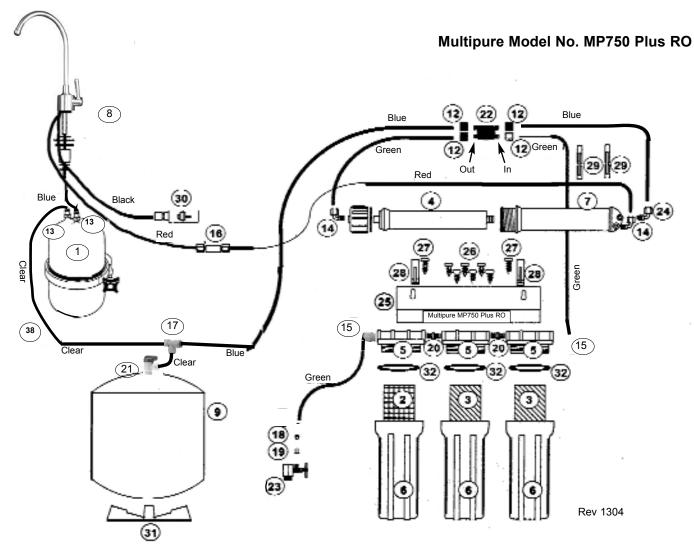
The reverse osmosis system contains a replaceable treatment component (Item #4), critical for the effective reduction of total dissolved solids. The product water should be tested periodically to verify that the system is performing properly.
